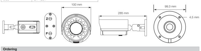
HCD95534X 1/3" CCD IR Bullet Camera, TDN, 530 TVL, 5-50 mm, 26 IR LED, PAL
